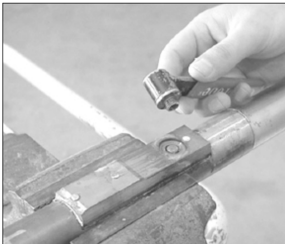
Figure 8.1: Unthread the membrane from the probe block.
