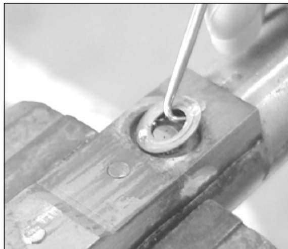
Figure 8.2: Remove and discard the copper washer.
